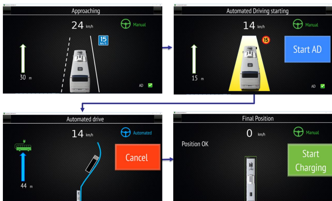
Figure 3. Linkker bus prototype HMI layouts: Approaching, Starting AD, AD and Final position.
